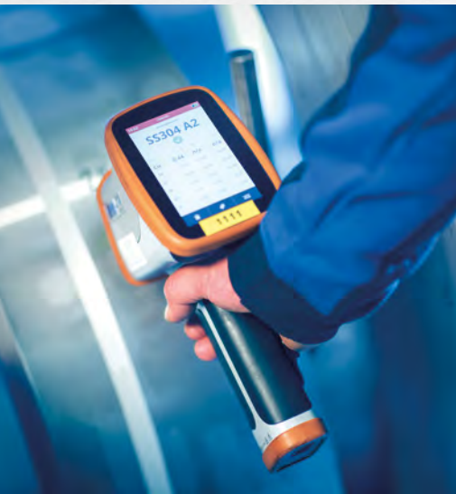
Quality control of the stainless-steel sheet material, using spectrum analysis.
