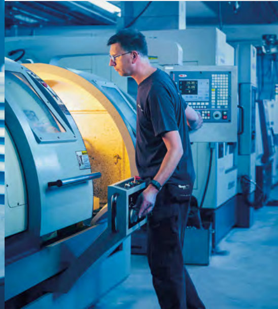
Parts for a new stainless steel die are being manufactured on the lathe.
