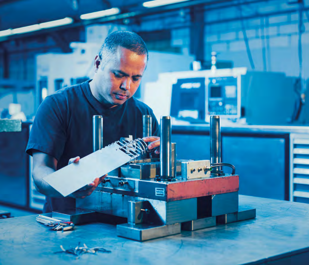
Inspection of a mould used to form the impeller vanes.
