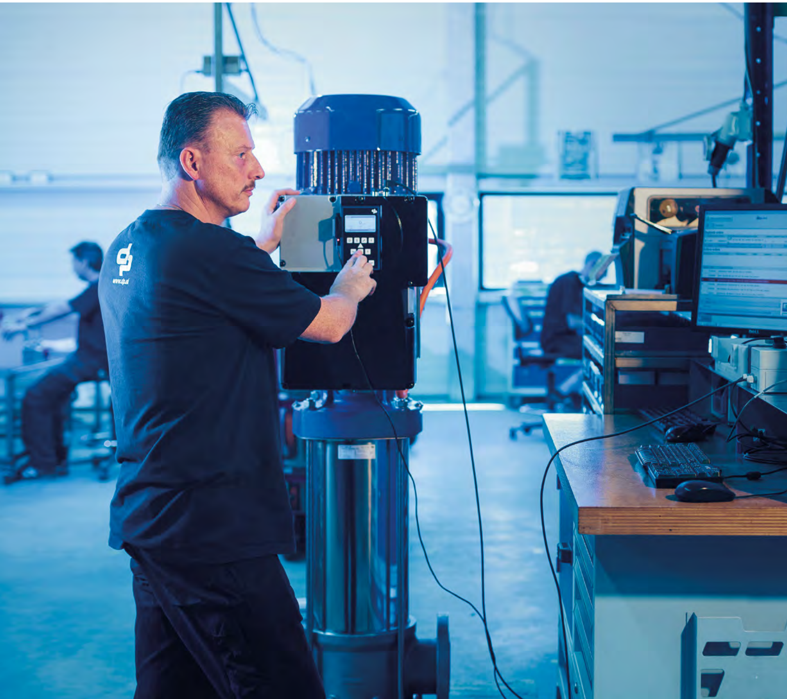
Pump and controls are attached to each other and tested.
