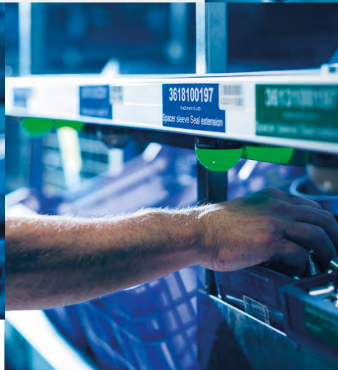
The assembly workers are directed to the correct parts using a pick-to-light system.
